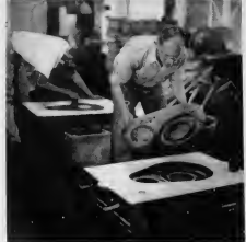
...splits the flask and removes the pattern ...habri e formalete y saca e pattern
